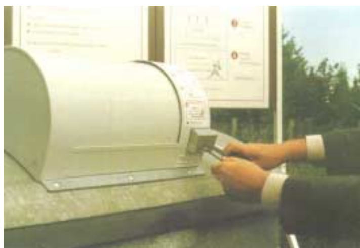
Figure 3: Display Showing Functioning of the Mechanical Lock gate: '(1) insert chip card (2) open gate (3) waste input (4) withdraw chip card'
